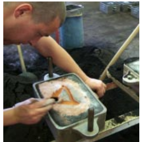
Aluminium casting, at Malmsteypan HELLA, photo taken for DVD presentation.
