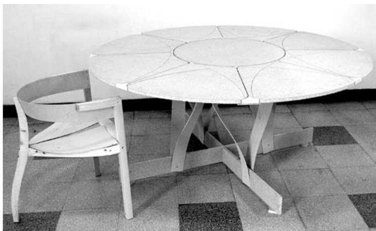
**Fig. 25 Steam bent leg table**
